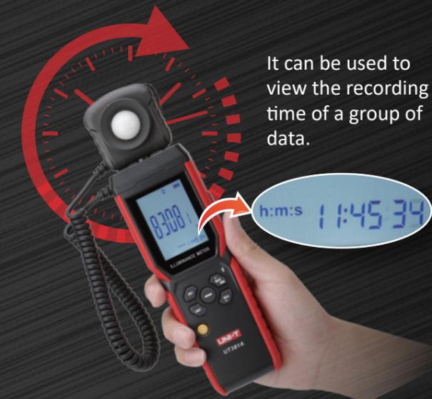
**Probe of integrated, split and rotatable design**
