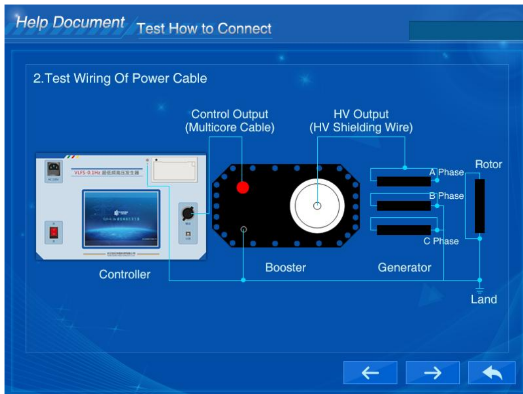
Figure 15 Wiring Diagram of Synchronous Motor
