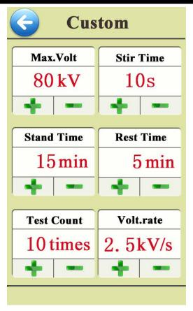
Voltage of boosting stop:  $10 \sim 80 \, kV$
