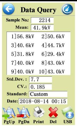
Click the "PgUp" or "PgDn" button to flip pages to display test data at different test times.
