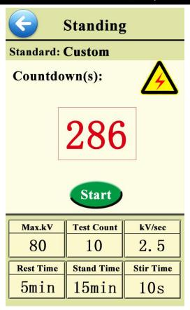
After the static time is over, enter the boost interface automatically. Click "st" button to skip the static entry and enter the boost interface. Click " to exit the test interface and return to the main interface.
