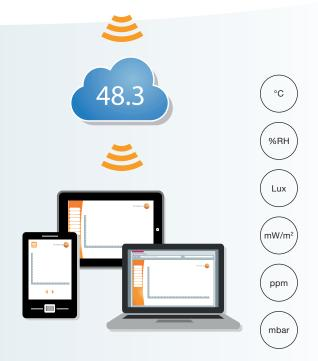
The monitoring system testo 160 monitors ambient conditions in display cases, exhibition rooms and depots. The loggers transfer measurement values by wireless LAN to the online store (Testo Cloud).
