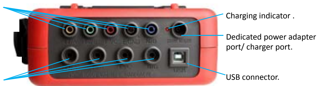
Figure 3-3: Connectors on the top of device
