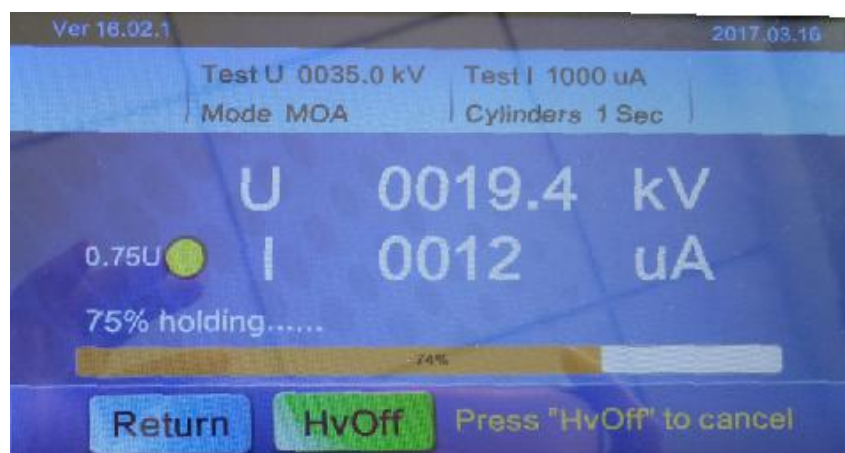
Figure 2-3.4-6 Holding Voltage of 75%
