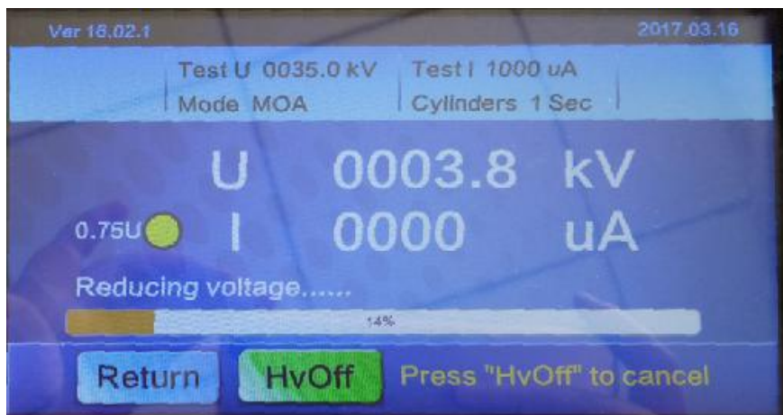
Figure 2-3.4-7 Voltage is Lowering Automatically
