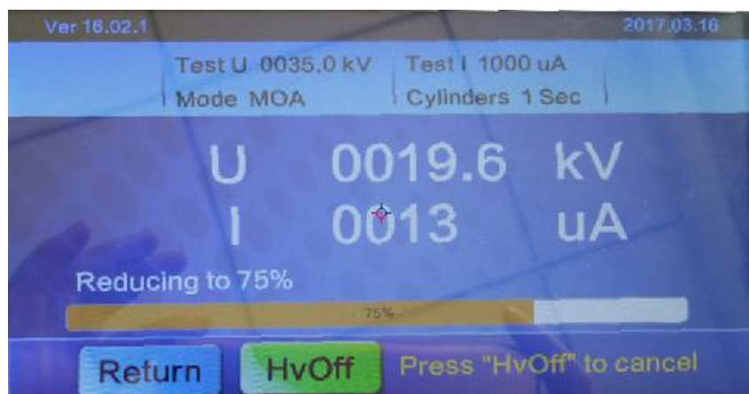
Figure 2-3.4-5 Voltage Drops to 75%
